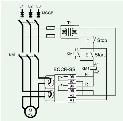
\* "N" (Fail safe) Type converts 95 → 96 to open and 95 → 98 to close when operating power is supplied to A1 and A2 (or L1 and L2).
