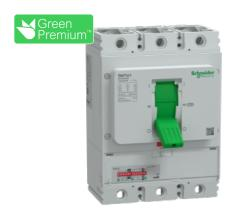
Circuit breaker, GoPact MCCB 800, 3 poles, 50kA at 415VAC, 500A rating, ETU trip unit, adjustable thermal protection
